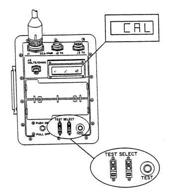
2-3-39. AC FREQUENCY 40 T0500 Hz (TEST PROBE) TEST #96
