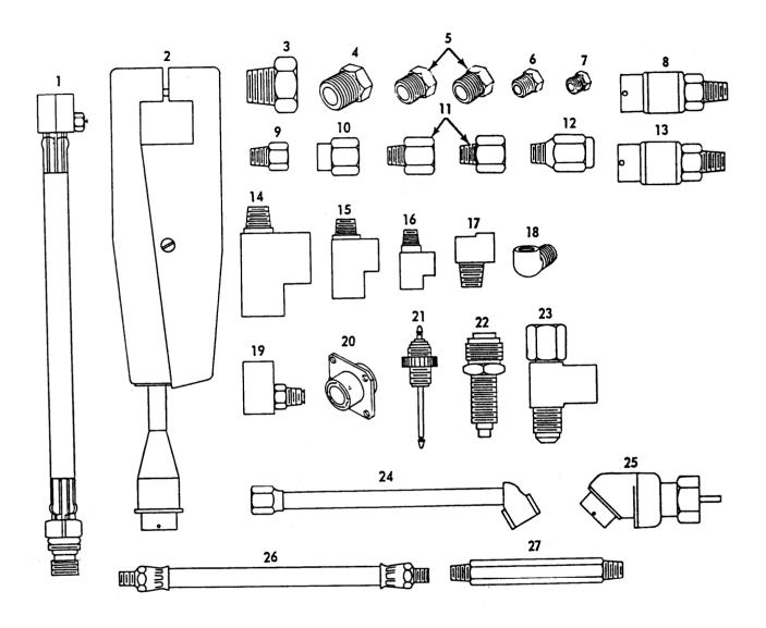
Figure 2. Transducer Kit (TK) Components.
