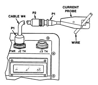
4. Attach current probe for single battery test. Clamp current probe around cable coming from positive (+) terminal of battery being tested. Point arrow on current probe along cable away from battery. Make sure current probe is closed. Go to step 7.
