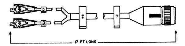
The power cable W5 is used to power the VTM when cable W1 is not being used. Cable W5 is divided into two leads with color coded clips, red for E1 and black for E2. Battery clips E1 and E2 are attached to a vehicle/equipment battery or to a 9 to 32 volt 4A regulated power supply. Do not connect the VTM to a battery charger unless it is also connected to a battery. Damage to the VTM may result.
