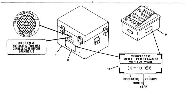
The STE/ICE-R set has only one instruction plate. This plate is attached to the STE/ICE-R transit case and contains instructions for the pressure relief valve. The instruction is as follows: RELIEF VALVE AUTOMATIC, TWO-WAY DEPRESS CORE BEFORE ENING LID.
