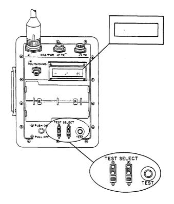
The diagnostic connector assembly (DCA) is mounted on a vehicle/equipment and allows the VTM to make measurements on the engine and accessories. The wiring harness for his connector is attached to a number of electrical test points and transducers inside the vehicle/equipment. This allows the user to determine the condition of chicle/equipment without disassembling the equipment to gain access.
