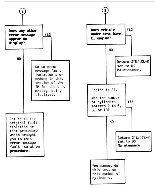
This message indicates that the equipment is not running or that the ignition adapter (TK item 30) is defective or missing.
