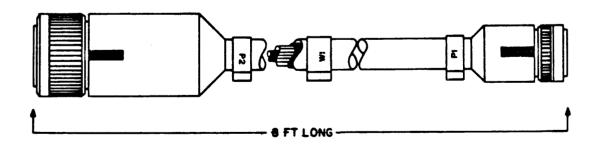
The DCA cable assembly W1 is used to power the VTM, and provides access to test points and sensors connected to the vehicle/equipment mounted DCA. When performing a DCA measurement, both the power and the measurement information are received through W1. For a measurement that is not DCA peculiar on equipment with a DCA, the VTM can receive power through W1, and use other cables to make measurements through the remaining connectors on the VTM.
