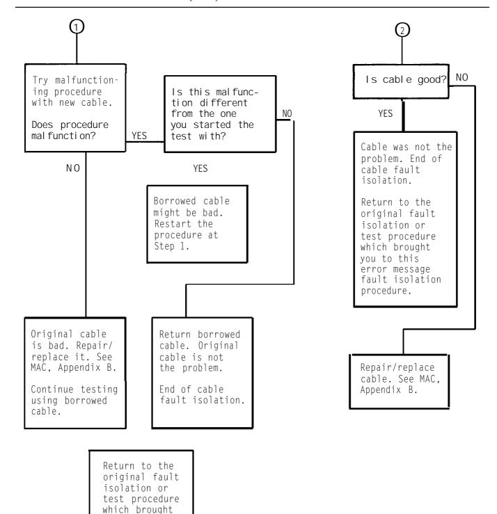
you to this cable fault isolation procedure.
