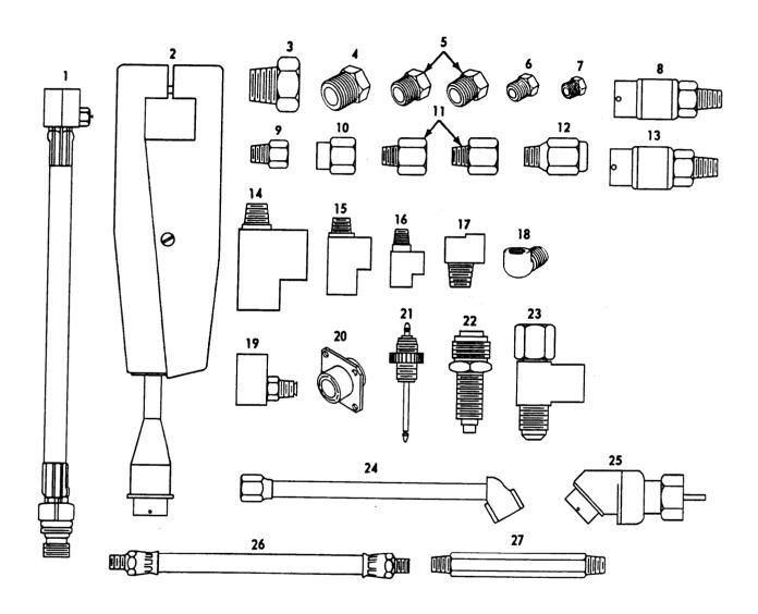
FIGURE 2. TRANSDUCER KIT (TK) COMPONENTS.
