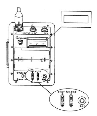
General measurements are those for which the VTM does not require a vehicle identification number in order to conduct the measurement. These include voltage, pressure, current, resistance etc. These measurements are useful in troubleshooting equipment such as air conditioners, electric generators, vehicles etc.
