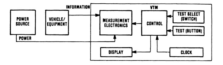
Setting the TEST SELECT switches to the required test number tells the VTM to make an RPM measurement when the TEST button is pressed and released.
