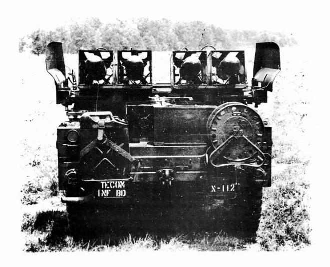
USATECOM PROJECT NO 8-3-4410-03 D, INTEGRATED ENGINEERING/SERVICE TEST OF THE ENTAC ATCM WITH MOUNTING KIT FOR M151,1/4-TON TRUCK
