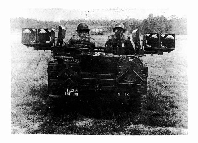
USATECOM PROJECT NO 8-3-4410-03 D, INTEGRATED ENGINEERING/SERVICE TEST OF THE ENTAC ATCM WITH MOUNTING KIT FOR M151, 1/4-TON TRUCK
